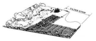
removing sediment and other pollutants from runoff as it flows through the filter strip. Some of the sediment and pollutants are removed by filtering, absorption, adsorption and settling as the velocity of flow is reduced.
