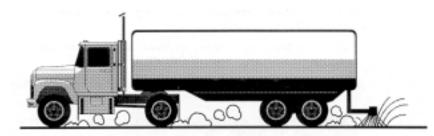
Reducing surface and air movement of dust from exposed soil surfaces during land disturbing, demolition, and construction activities.
