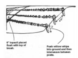
Spaces between the woven "fences" are filled with topsoil. Fences are generally arranged parallel to the slope or in a grid pattern diagonal to the direction of the slope.
