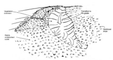
stable areas without causing erosion. It allows concentrated runoff to be discharged at non-erosive velocities onto natural or man-made areas that have existing vegetation capable of preventing erosion. An example would be at the outlet of a diversion or a waterway.
