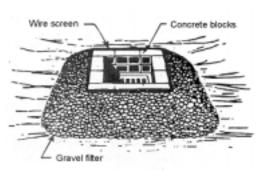
Concrete blocks are laid without mortar closely around the perimeter of the drain. Gravel is then placed around the outside of the blocks to restrict the flow and form a sediment pool. For slower drainage and therefore more settlement time, the concrete blocks could be eliminated and the device made entirely of gravel.
