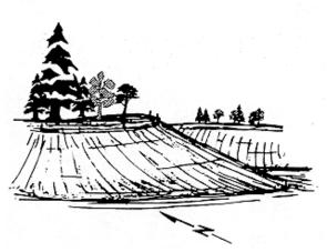
erosion is magnified. Swales and channels concentrate surface flow, which results in higher velocities. Exposed south-facing soils are hotter and drier, which makes vegetation more difficult to establish.
