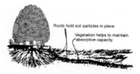
Vegetation slows the velocity of runoff and acts as a filter to catch sediment.
