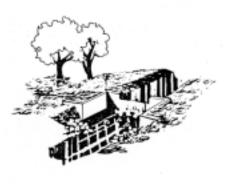
of flow, therefore, special care must be taken to prevent undercutting at the toe of the structure and erosion of the banks.
