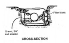
around the pipe. Manufactured filters designed for the purpose, such as filter fabric, may be used as alternatives.
