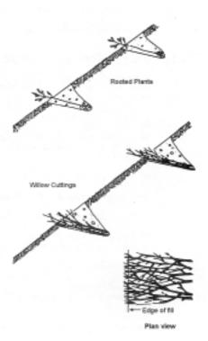
reinforcing units. The portions of the brush that protrude from the slope face assist in retarding runoff and reducing surface erosion.
