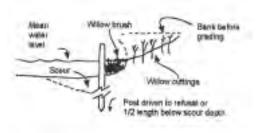
Fasten heavy wire fencing to the post and if the streambed is subject to scour, extend it horizontally on the streambed for a distance equal to the anticipated depth of scour and weight with concrete blocks. As scour occurs, this section will drop into place.
