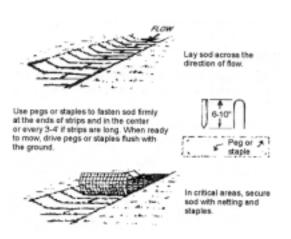
pegged over the sod for further protection against washout during establishment.
