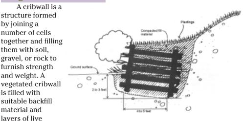
branch cuttings. The cuttings root inside the crib structure and extend into the slope. Once the live cuttings root and become established, the subsequent vegetation gradually takes over the structural functions of the wood members.
