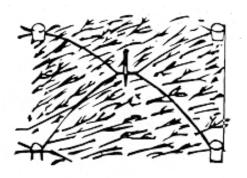
Many types of mulch are available; such as straw, woodchips, and excelsior mats. Most mulches must be anchored, using plastic emulsions or jute, fiberglass, or plastic netting.
