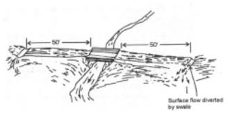
water from flowing along the roadway and directly into the stream.
