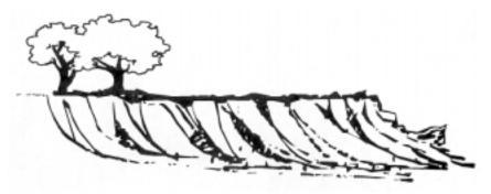
Soil erosion, aesthetics, and adverse impacts on water quality are concerns associated with the operation, maintenance, and closure of sand and gravel pits. A good vegetative cover of grasses and legumes can alleviate these concerns. Vegetative cover will retard surface runoff and prevent erosion, reducing the sedimentation of nearby streams, waterways, and waterbodies. Vegetative cover will enhance the aesthetics of sand and gravel pits while providing nesting and escape cover for wildlife.
