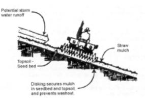
Temporary seeding controls runoff and erosion until permanent vegetation or other erosion control measures can be established. Root systems hold down the soils so that they are less apt to be carried offsite by storm water runoff or wind.
