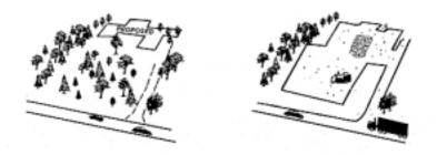
Changes in drainage areas caused by regrading the terrain, diversions, or road construction.
