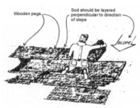
Waterways carrying intermittent flow: where immediate stabilization or aesthetics are factors; where velocities will not exceed that specified for a grass lining; and other locations which are particularly suited to stabilization with sod.
