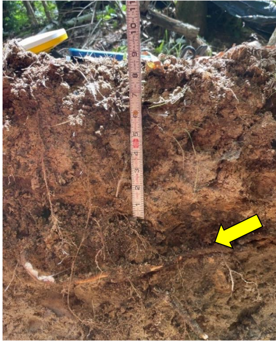
Photo 1 View south of Test Pit #1 in Trench 1. The buried topsoil visible on the south side of the trench was observed approximately 8 inches from the soil surface (6/22/23).
