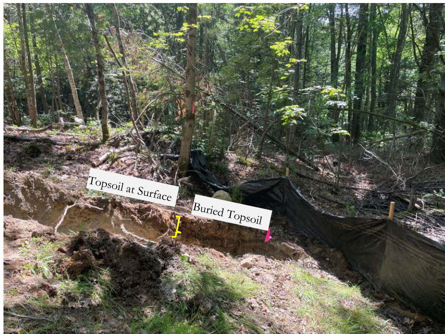
Photo 2 View south of the Trench 1 where topsoil transitions from at the ground surface to being buried (6/22/23).
