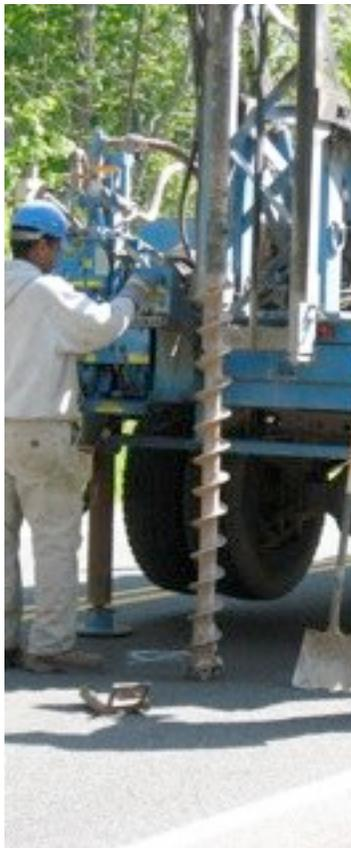
The crew from Seaboard Drilling Company worked with our environmental scientist, Joel Harris, to take numerous samples at different depth. We were surprised to be able to drill to 14' without hitting any bedrock. We hit bedrock at 2 other locations during the big dig and there have been many stories of bedrock being hit over the years and during the LCP road project. Five samples were taken and did prove to show contamination at 6-8'.
