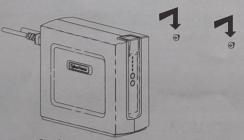
Use the enclosed wall mount template to locate screws on the wall. Hang the DTC36U12V on the screws which are located on the wall
