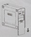
a. Slide off the battery cover at the back of the DTC36U12V unit.
