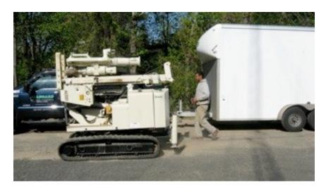
Three samples were dug into the floor of the fire station. The one near the ball field hit ledge at three feet and was fine. The second in the large bay was okay. The sample dug in the north rescue bay was not good at a depth of 6-8 feet. This is near where the tank had been removed and pump is suspected of leaking.
